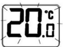
You can change the set point temperature very easily while you are reviewing the set point temperature. Press the UP or DOWN keys repeatedly to change the temperature setting. The set point temperature will flash to indicate that it can be changed:
