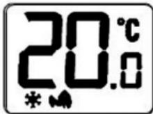
Whenever Frost Protection is activated, the Frost Protection indicator will flash in the sequence shown below:
