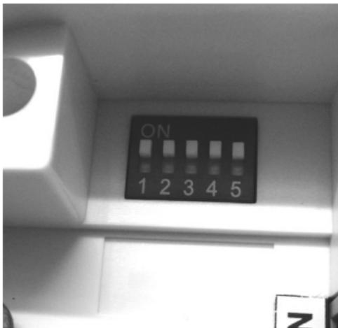
To adjust the RF address code of the Control Centre, remove one or more of the jumper caps located on the back of the unit (labelled 5,4,3,2 and 1, and shown in the picture below) so that the jumper settings match the settings made on the receiver:
