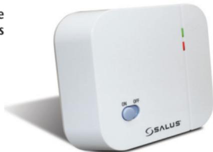
On the front cover of the Receiver you will see that there is the On/Off switch and two Light Emitting diodes (LEDs). The switch allows you to turn off the Receiver if necessary to prevent it calling for heat. The bottom LED (red) will illuminate when the switch is in the 'On' position and the unit is receiving power. The top LED (green) illuminates when the Receiver unit is receiving a heat call transmission from the Control Centre.
