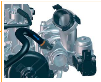
Non-Return Valve Intake Side on the Exhaust Gas Turbocharger
