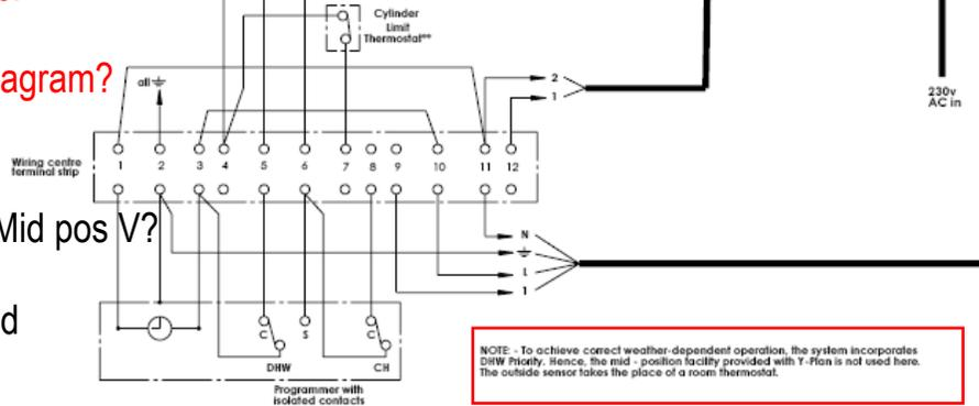
NOTE - To achieve correct weather-dependent operation, the system incorporates DHW Priority. Hence, the mid - position facility provided with Y-Plan is not used here. The outside sensor takes the place of a room thermostat.
